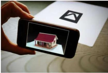
Figure 1. Example of AR Marker Based Tracking [6]
