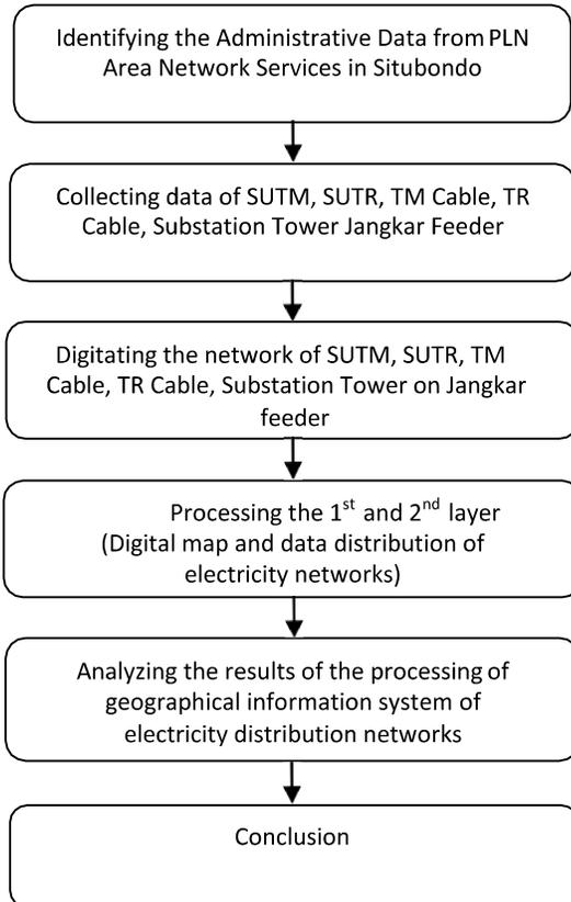
Figure 2. Flowchart of mapping the electricity distribution network
