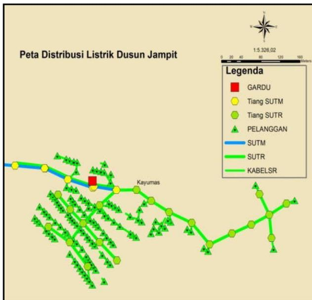
Figure 7. The Mapping of SUTM and SUTR in LD197 Substation
