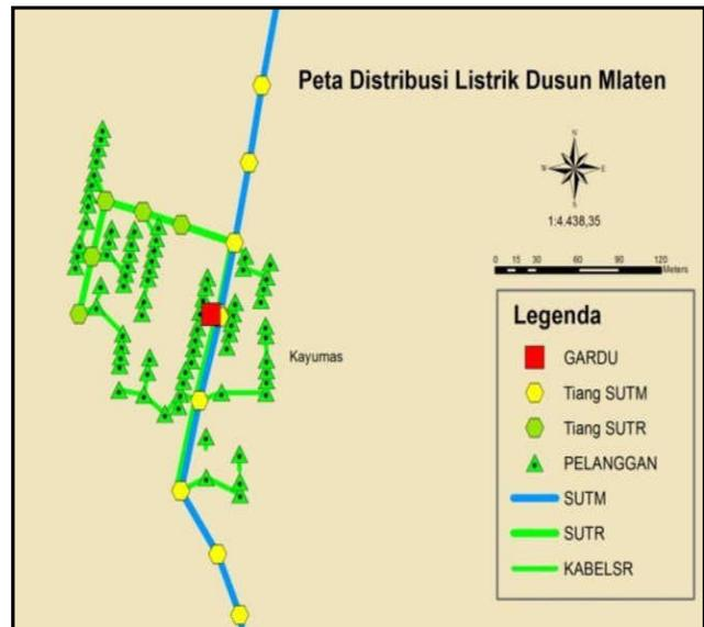
Figure 6. The Mapping of SUTM and SUTR in LD196 Substation
